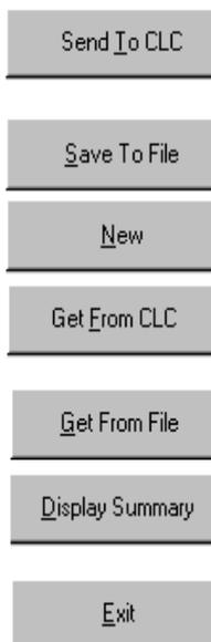
**Send To CLC** Saves the currently selected object mapping list to the CLC-D Card (to card parameter C-0-2600 if the cyclic [PD] channel is selected, and C-0-2700 if the non-cyclic [PCP] channel is selected).
