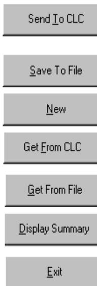
Saves the currently selected object mapping list to the CLC-D Card (to card parameter C-0-2600 if the cyclic [Polled I/O] channel is selected, and C-0-2700 if the non-cyclic [Explicit Messaging] channel is selected).
