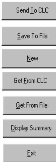
Saves the currently selected object mapping list to the CLC-D Card (to card parameter C-0-2600 if the cyclic [DP] channel is selected, and C-0-2700 if the non-cyclic [FMS/P-Chan] channel is selected).
